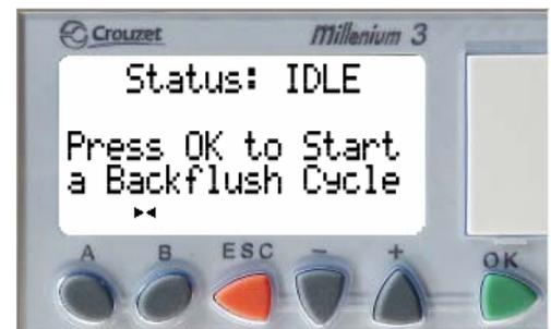
When the pressure differential set-point is reached, the controller will display **High Press. Diff.!** for a period of time (typically 5 seconds) before initiating a backflush cycle. The controller will automatically display the status screen if a backflush cycle is initiated or if the pressure differential set-point is reached.
