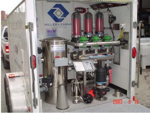
Miller-Leaman's fully operational trailer; used for demonstration and water testing purposes
