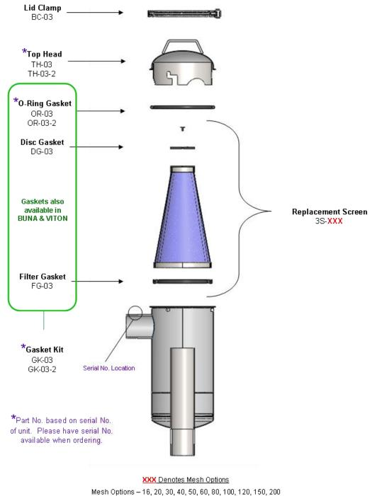
Heavy Duty Mesh – 24x110, 30x150, 40x200, 50x250 (Dutch weave screens; heaver wire gauge, lower open area %)
