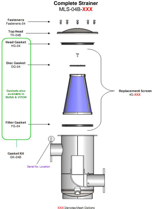
Mesh Options – 16, 20, 30, 40, 50, 60, 80, 100, 120, 150, 200 Heavy Duty Mesh – 24x110, 30x150, 40x200, 50x250 (Dutch weave screens; heaver wire gauge, lower open area %)
