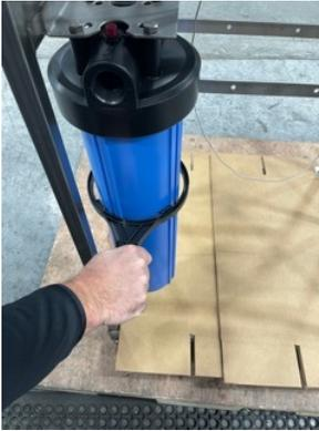
**STEP 4-Using Provided Housing Wrench, Remove Filter Housing**
