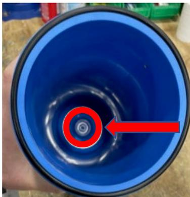
**STEP 6- Place new Filter in Housing Ensuring the Filter is lined up with the Nipple on bottom of Filter Housing**
